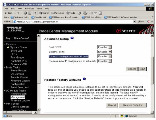
Figure 5-3 Enabling management over all ports using the Management Module Web interface
